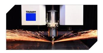
Our latest fibre laser cutting technology has capabilities to laser cut copper up to 8mm in thickness. Together with enhanced deburring equipment and our in house electroplating, we produce highly toleranced parts and sub-assemblies.
